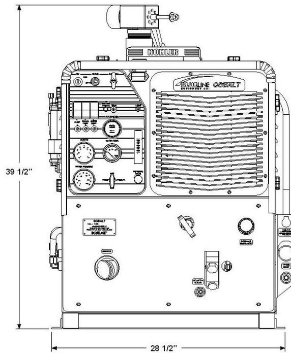
**DIMENSIONAL DIAGRAM w/ SUB-MOUNT WATER TANK**
