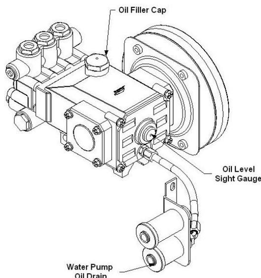
2. After the first **50 hours** of operation, change the crankcase oil with CAT Pump Crankcase Oil, (Part # 13-000). Change the crankcase oil every **500 hours** thereafter.
